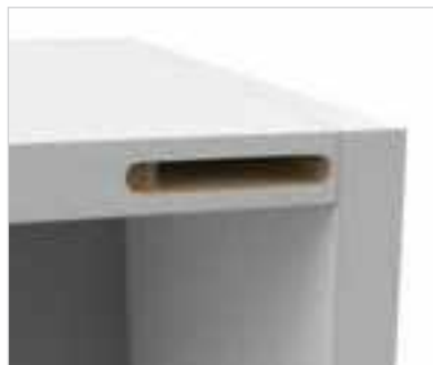
7. Make cavities according to the technical specifications for the Klar hinge body in the top and bottom panels of the cabinet.
